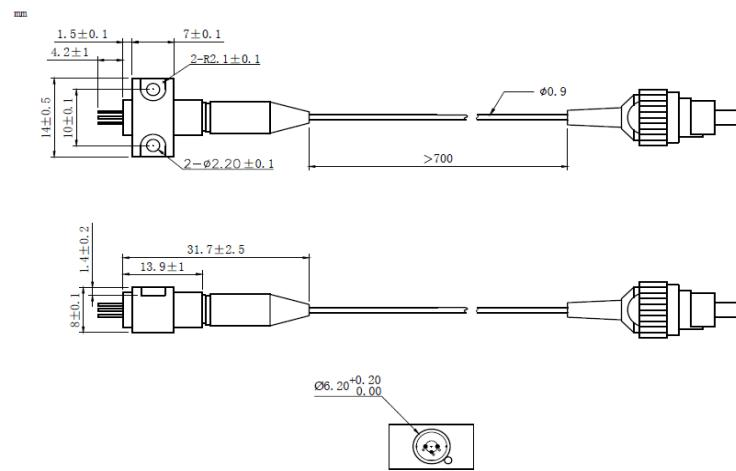
**8-Pin Package View (built-in TEC) :**
